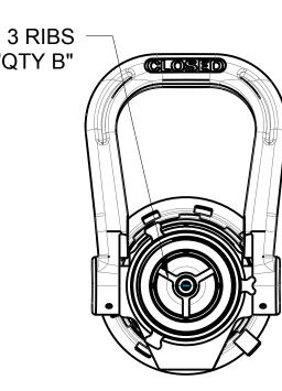
WHEN VIEWING INTO NOZZLE THROUGH THE SWIVEL NOTE THE NUMBER OF RIBS ABOUT THE CENTER. IF THERE ARE 2 USE COLUMN "QTY A". IF THERE ARE 3 USE COLUMN "QTY B".
